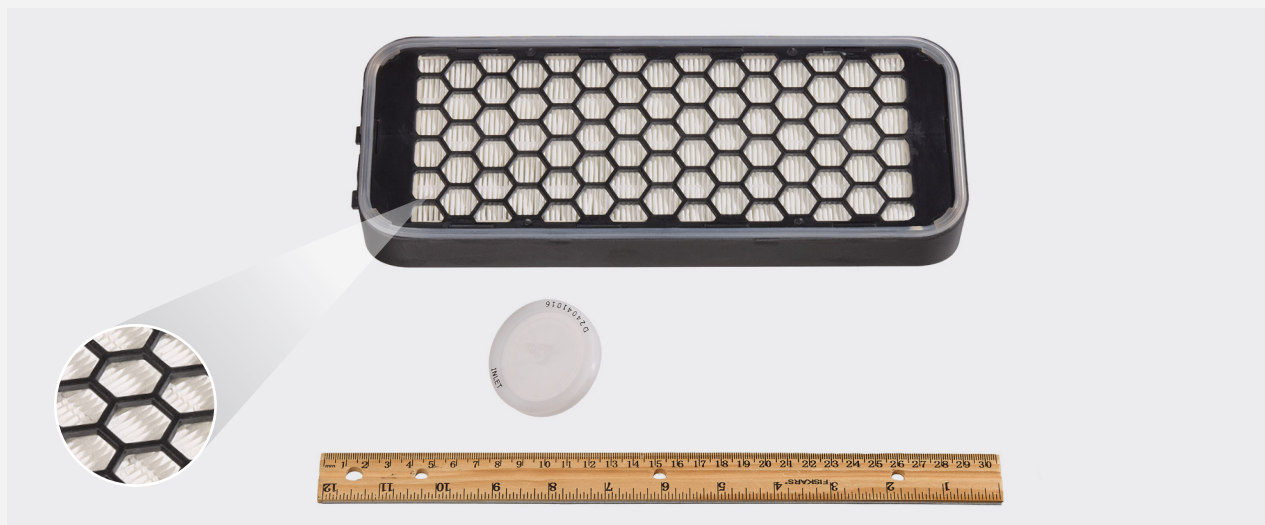
Figure 4: Side by side comparison. A three-dimensional, pleated depth HEPA filter (top) next to a two-dimensional membrane disk air filter (below). Zoomed in view shows the three-dimensional mesh structure of the HEPA filter and indicates why a circulating fan is required to force air through the fibers
