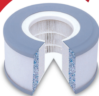
Figure 1: A HEPA filter with a cutout showing the three-dimensional depth structure of the filter medium. This example also includes a molecular sieve medium to capture volatile organic compounds (VOCs).
