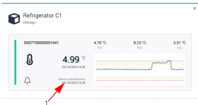
Figure 30. Sensor details panel showing alarm pause is activated on the data logger
